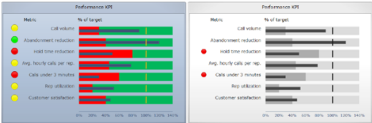
Figure 3. Left: an example of the overuse of both color and alerts. Right: an example of a better design (example Few, 2013).
