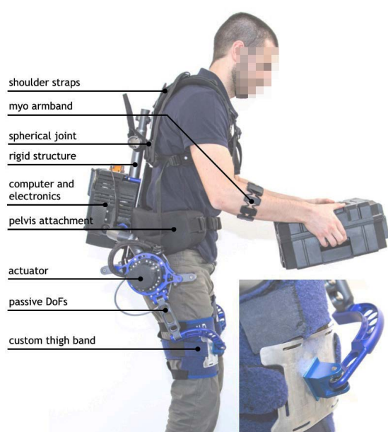
Figure 1. Side view of the back-support exoskeleton prototype (DoF stands for Degree of Freedom).
